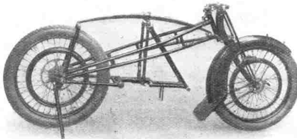
Details of the spring frame construction of the McKechnie Motor-cycle.
