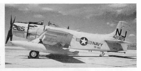
At right, an AD-7 Skyraider with wing tanks, empty rocket racks, and looking remarkably clean. Note, the different cockpit canopy shape to the AD-5 opposite.
