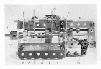
A 4-speed Gearbox with a gate change built by—we don't know who! Owing to internal reorganisation, all correspondence relating to the mechanism has been lost so, if you built it, please write to Spanner.
