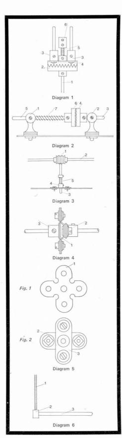
Handrail Support 1, on the other hand, is a 1½ in. Rod 5 that carries another ½ in. Contrate Wheel 6 on its inside end with a Compression Spring 7 between the Contrate and the Handrail Support. The Compression Spring keeps Contrate 6 in mesh with Contrate 4.
