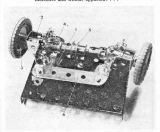
The free ends of the Universal Couplings at each side are now joined by a  $1\frac{1}{2}$  in. Rod centrally journalled in a Stepped Bent Strip 5. A  $\frac{1}{2}$  in. Pulley with boss is fixed on the Rod between the lugs of the Bent Strip, as shown, then two Fishplates are bolted one to the rear lug of each Double Bent Strip 1. To complete the unit, a  $2\frac{1}{2}$  in. Strip 6 is lock-nutted between these Fishplates.
