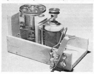
The upper winch house is constructed around a base of  $\frac{1}{4}$  in. ply. A ply base 4 in.  $\times$  2 in. will be large enough to accommodate a suitable size of electric motor. A front panel, also in  $\frac{1}{4}$  in. ply, is cut to a size of 2 in.  $\times$  1 $\frac{3}{4}$  in. and screwed to the end of the base with woodscrews. Two side pieces are then cut from  $\frac{1}{8}$  in. ply to a size of  $4\frac{1}{4}$  in.  $\times$  1 in. and again screwed in place, as shown.
