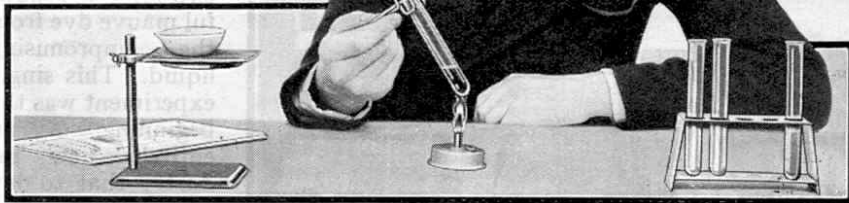
Fig. 1. A well-arranged experiment. The Test Tube in which a solution is being prepared is held in the correct position, with its mouth pointing away from the face, and the rest of the apparatus is within easy reach, but is not in danger of being accidentally knocked over.
