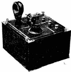
A COMPLETELY ASSEMBLED POLAR BLOK CRYSTAL SET IN A POLISHED WOOD CASE
