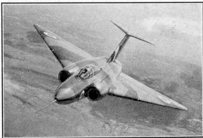
A striking view of the Gloster Javelin two-seat delta fighter. Photograph by courtesy of the Hawker Siddeley Group Ltd.
