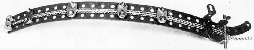
Below: Fig. 23: Chain guide from the north, showing chain location, also details of station and pusher.
