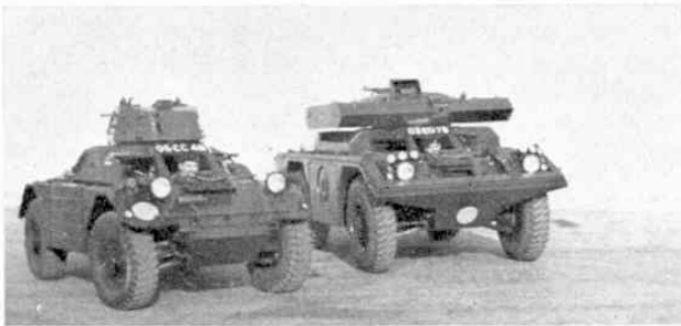
Scout car development; two versions of the Ferret, one with small open machine-gun turret, the other with anti-tank missile pack.
