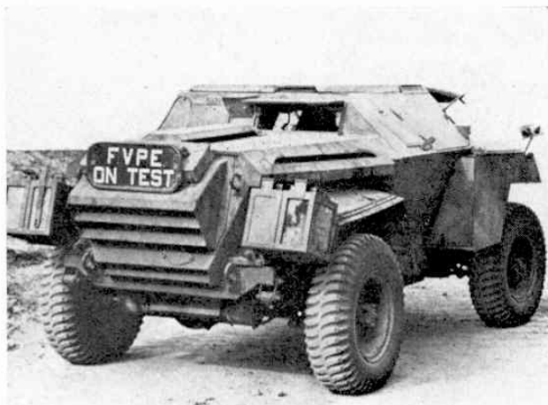
Left, British Scout Car, WWII, built by Humber, seen from the rear. Angled hull for maximum protection, open top (no turret) and rear engine.
