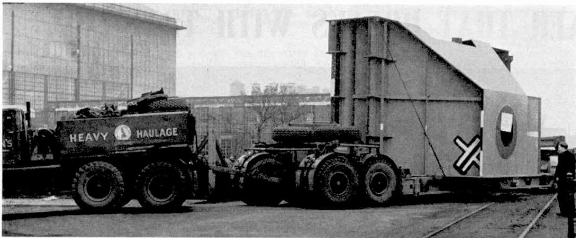
The largest single unit of the dragline, weighing 42 tons, leaving the works on a low-loader.
