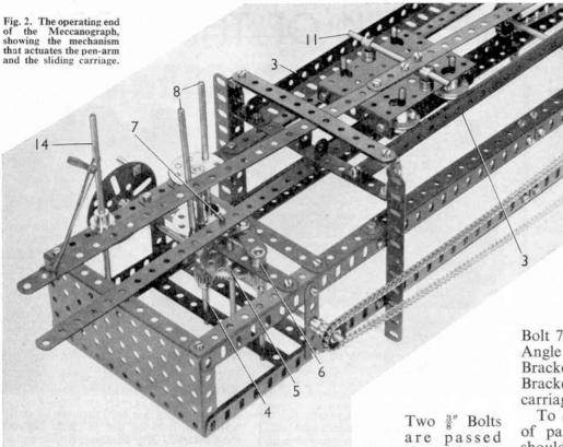
Plate and the Double Angle Strips as shown, and each of them carries a 1" Pulley and a Spring Clip. The boss of each Pulley is spaced from the Flanged Plate by two Washers.
