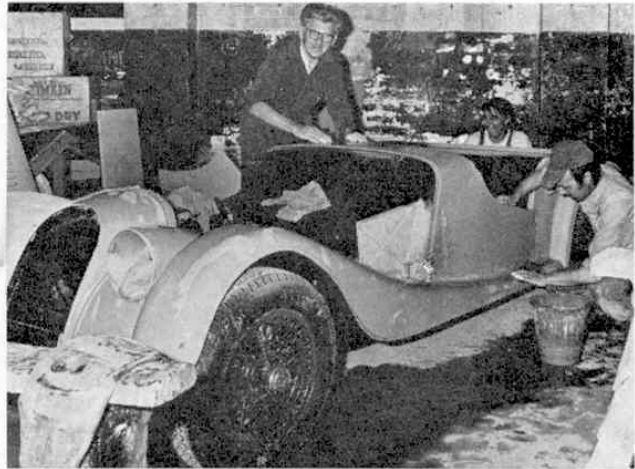
Rubbing down the bodywork of a Morgan 4/4 before spraying.
