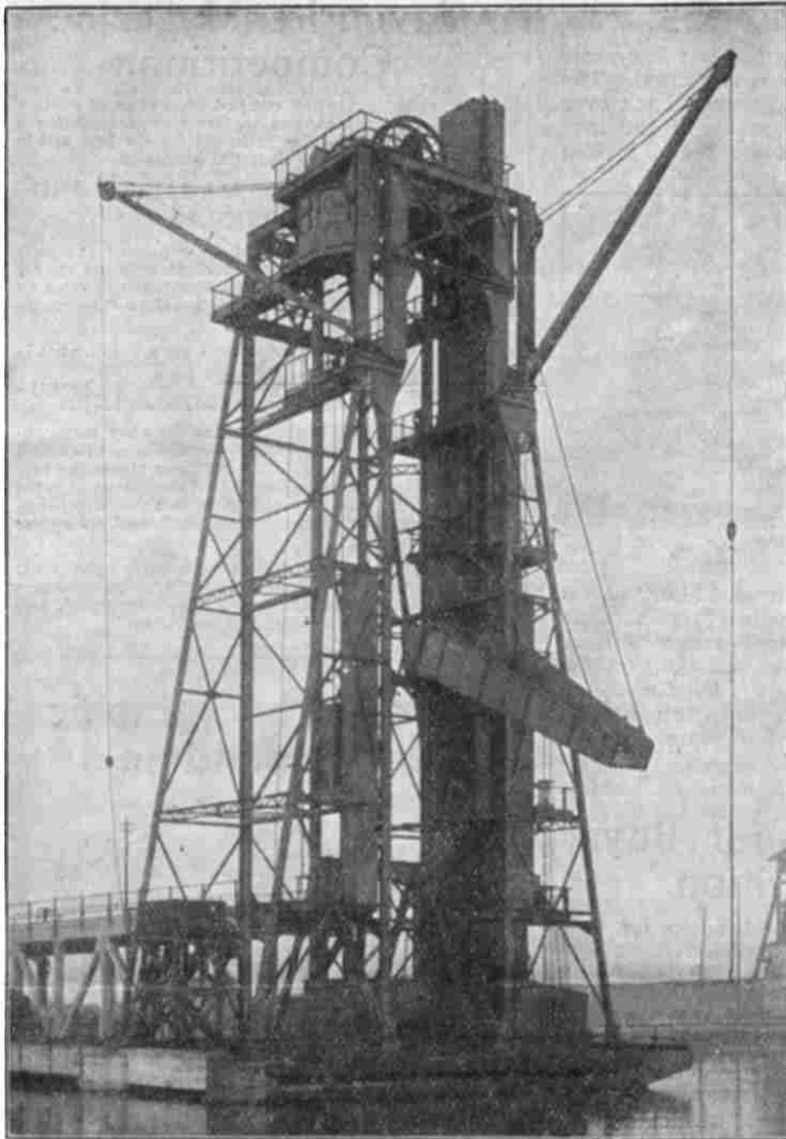
This Hydraulic Coal Hoist lifts a full truck of coals, weighing 30 tons, to a height of 60 ft.
