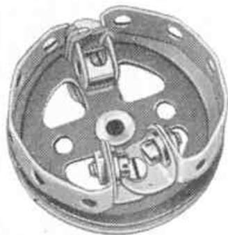
Fig. 1. The internal expanding brake fitted to the driving wheel of the truck.
