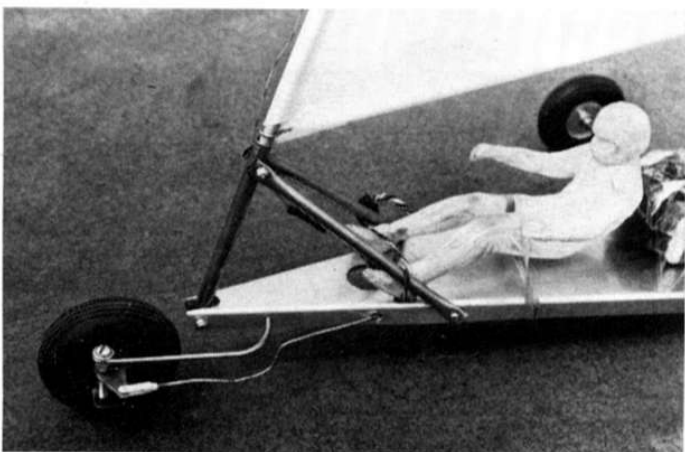
Below left, an underside view showing the installation of simple radio; the battery is carried above the chassis. Right, basic mast support and steering arrangement.
