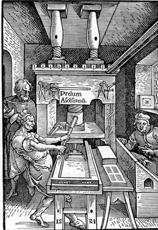
An interesting old woodcut, showing the interior of a printing works in the early 16th century. An impression from type set up by the compositor on the right is being pulled on the crude but powerful press, and on the left is a man with ink swabs waiting to ink the types.
