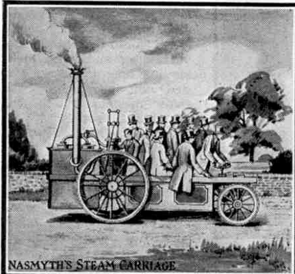
A steam-driven road carriage built about 1827 by James Nasmyth, the famous engineer. It was capable of conveying eight persons.
