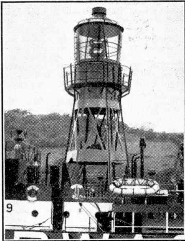
A close-up of the lantern in a modern lightship. Photograph by courtesy of Philip and Son Ltd.
