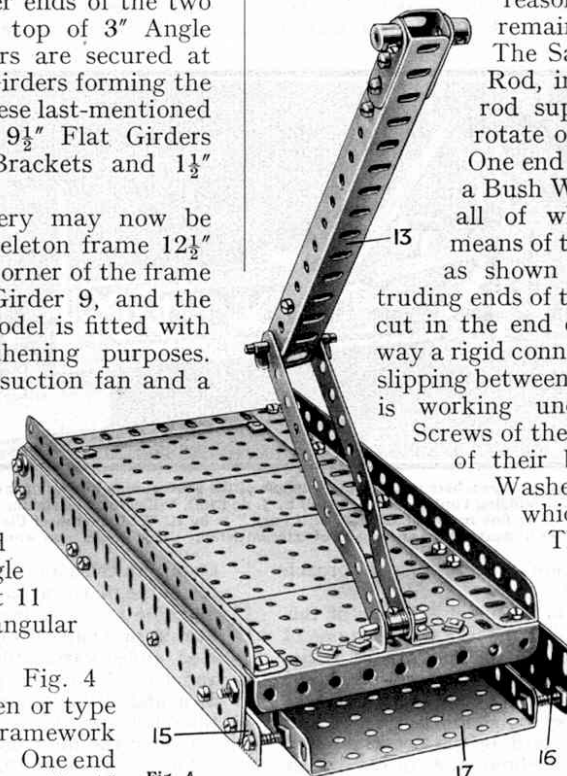
Fig. 4. This underneath view of the platen shows its construction and also the method of operation.
