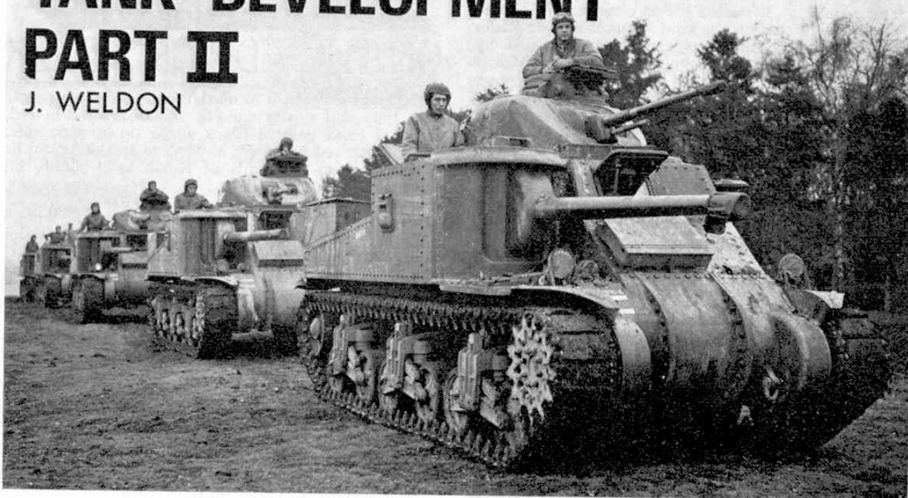
This was the American M3, known as the 'Lee' (American turret) or 'Grant' (British turret). Comparison with the Soviet T34/85 shows it as an inferior machine in that its silhouette is higher; the main armament is not in the turret; construction is by riveting, not cast or welded.
