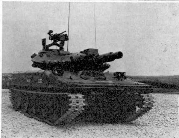
Above: The M60, the U.S. equivalent to the "nuclear age" Chieftain. Note the night navigation and range-finding equipment.
