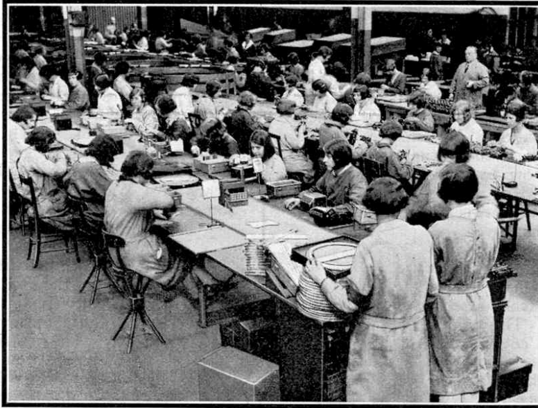
The system of line conveyor work is made clear in this photograph. On the nearest belt a variety of articles are being assembled, including turntables, signal boxes, level crossings and locomotive tenders. The assembly of locomotives is in hand on the second belt. The test tracks referred to in the article are plainly shown.
